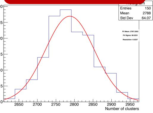
Resulted in improved dN/dx resolution: from 2.38% to 2.28% fo 2-meter tracks
