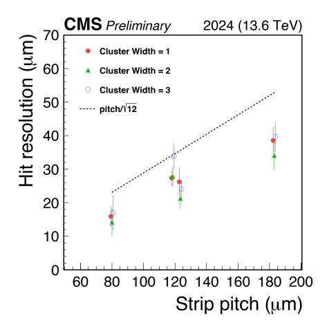
Strip hit resolution is derived by selection pairs of hits in different types of overlapping sensors and for different cluster widths expressed in units of number of strips
