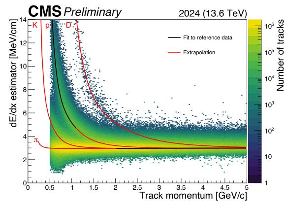
Energy loss measurement as a function of the track momentum using the Pixel-Less Harmonic-2 estimator. The data were fitted on the shown proton and pion band using the function
