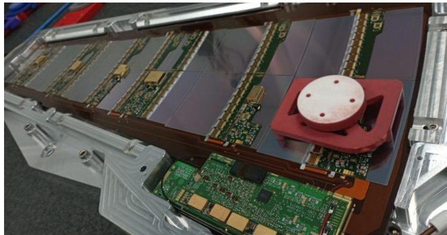
Load modules to stave/petal via silicone
