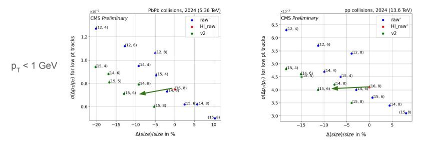
The configuration for barycenter, and average charge (15,6) in v2 gives reduction in strip cluster collection's size > 10% with respect to current method, while keeping similar performance in track reconstruction.
