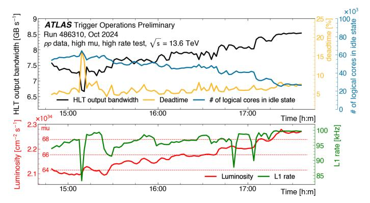
\* dead-time used to prevent buffer overflows in the front ends.
