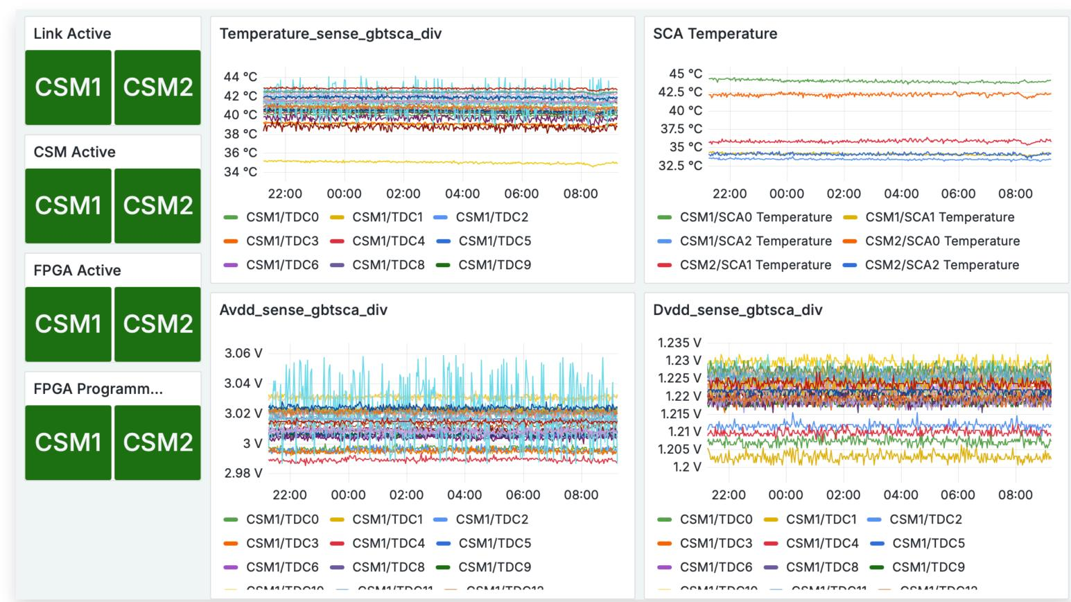
with the ATLAS Detector Control System etector electronics
