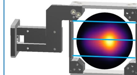
Fibers measure circulating beam fast rotation intensity
