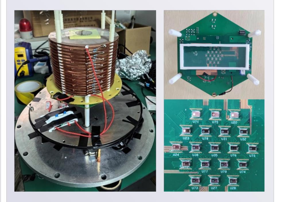
•SeF high electron affinity  $\rightarrow$  negative ions are drifting  $\rightarrow$  new sensor developed to detect negative ions and achieve good energy resolution without electron avalanche multiplication
