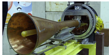
Polarised target refrigerator and MW cavity.
