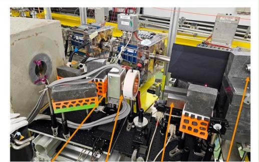
Sapphire detectors YAG screen W collimator camera
