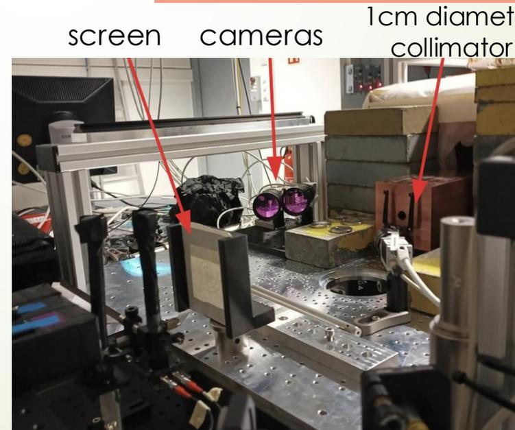
High flux laser-plasma test beam at DESY
