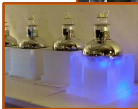
Optical Module (OM): Polystyrene scintillator + PMT
