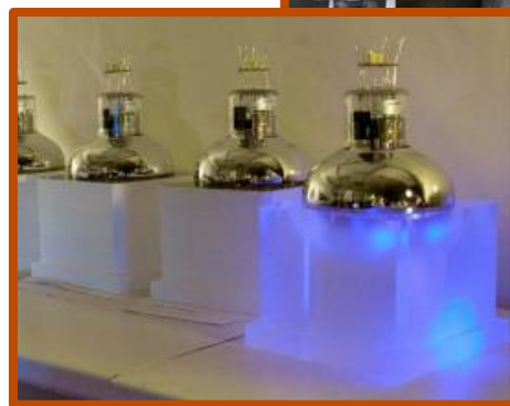
Optical Module (OM): Polystyrene scintillator + PMT
