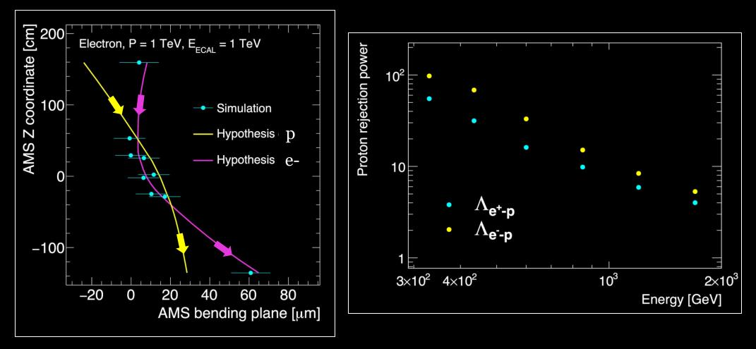
Parameters from competing track fits along with event characteristics in tracker and TOF (charge, noise) are used to construct multivariable estimator providing an independent from TRD and ECAL suppression of the proton background at TeV scale.
