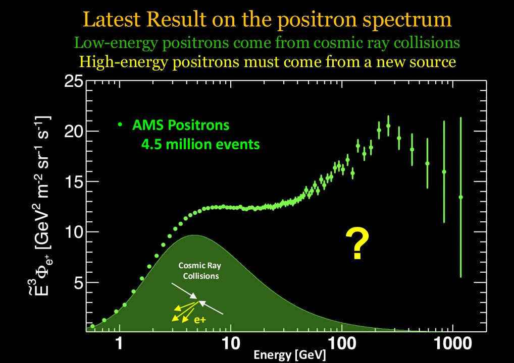
The positron flux is the sum of low-energy part from cosmic ray collisions plus a high-energy part from pulsars or dark matter with a cutoff energy
