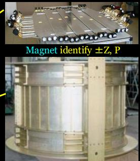
Anticoincidence Counters (ACC) reject particles from the side
