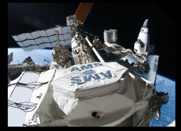
AMS on ISS provides long term precision measurements of charged cosmic rays. Research topics: the Origin of Cosmic Rays, Physics of Dark Matter and Antimatter.
