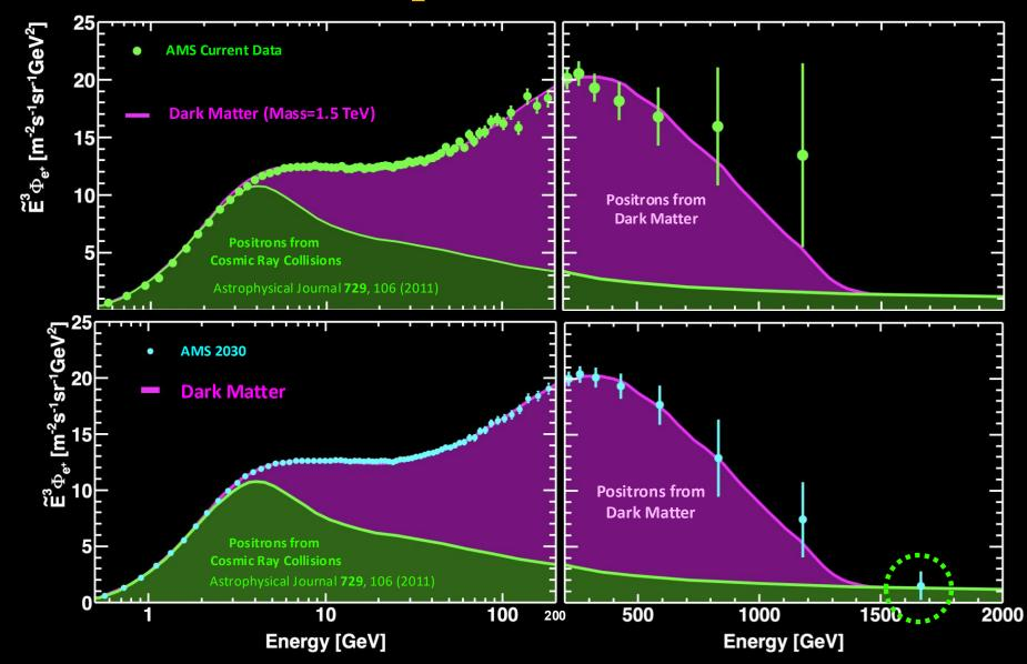
By 2030, AMS will ensure that the high energy positron spectrum drops off quickly in the 0.2-2 TeV region and the highest energy positrons only come from cosmic ray collisions as predicted for dark matter collisions
