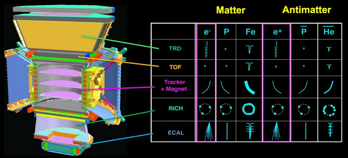
In 13.5 years, the detectors have performed flawlessly. AMS is able to pick out 1 positron from 1,000,000 protons; unambiguously separate positrons from electrons up to a trillion eV; and accurately measure all cosmic rays to trillions of eV.
