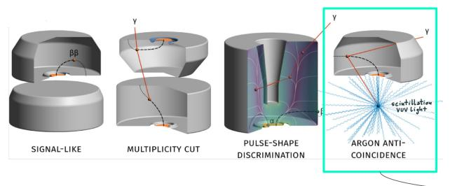
Instrumented **LAr** (fibers, SiPMs) detects **scintillation light** when some energy is released in argon in coincidence with an energy deposition in germanium.
