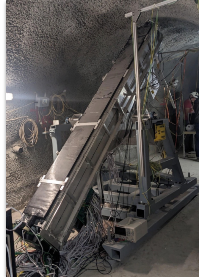
4 supermodules (64 bars) put into the cage to make the final bar detector
