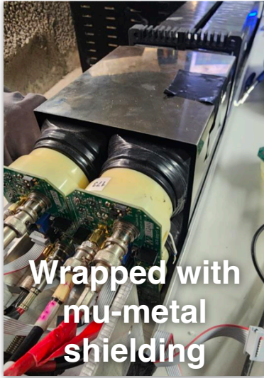
4 bars assembled into an unit
