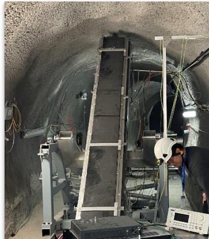
4 supermodules (64 bars) put into the cage to make the final bar detector
