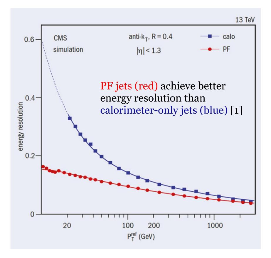
In CMS, PF algorithm is crucial for physics measurements—significantly improving jet energy resolution over local reconstruction algorithms
