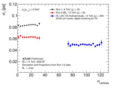
Time resolution of  $B_s \rightarrow J/\psi \phi$  for different numbers of reconstructed PV in the same bunch crossing PubNote
