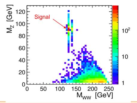
MC studies indicates that observation of the new scalar production through the scalar-strahlung process with decay to W+W- should be feasible at a 250 GeV Higgs factory for scalar masses between 125 and 150 GeV
