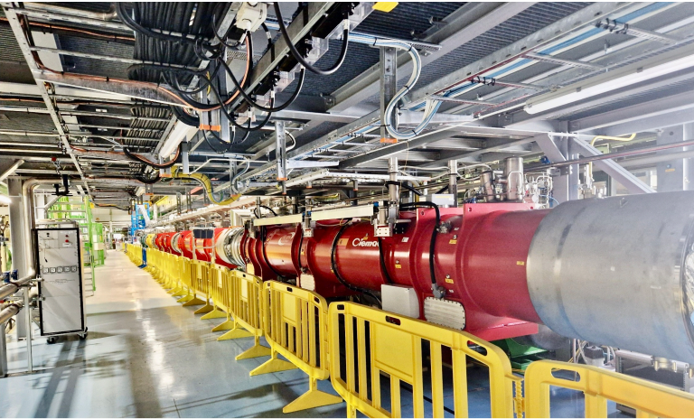
Fully realistic inner triplet string test facility at CERN, from left to right: installation of superconducting link, installation of D1 and Q2a cryo-assemblies, tests to start in Oct 2025
