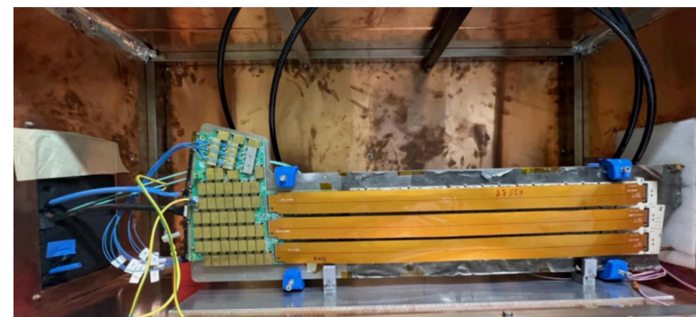
HGTD LGAD sensors in production, continued tests with demonstrator
