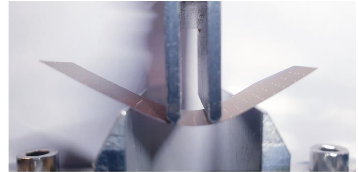
Figure 4.41: Setup for the bending strength measurements.
