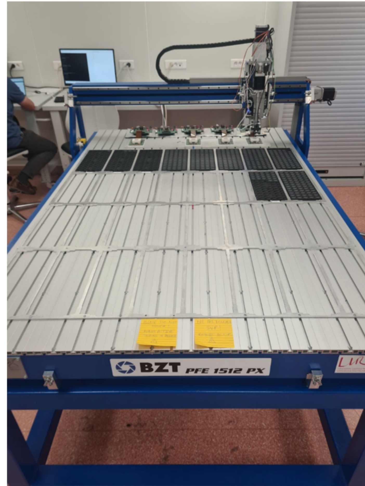
Figure 12: HGCROC robotic testing facility at LLR.
