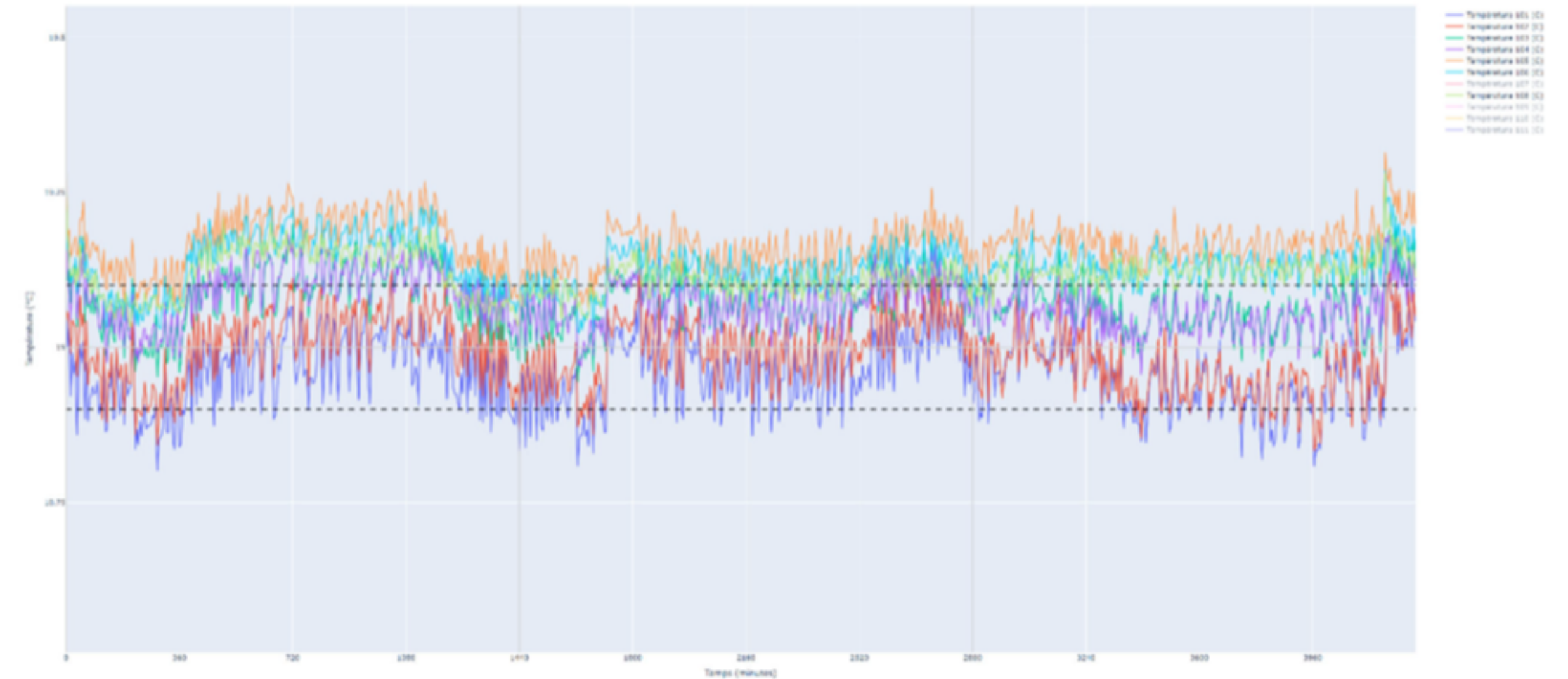
Figure 14: Temperature measured as a function of time at different positions across the PWO crystals during the beam-test measurements at CERN with the 5x5 EEEMCal prototype.
