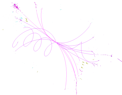
Figure: The reconstructed PFOs in an event of E_{\text{CM}} = 91.2 GeV.
