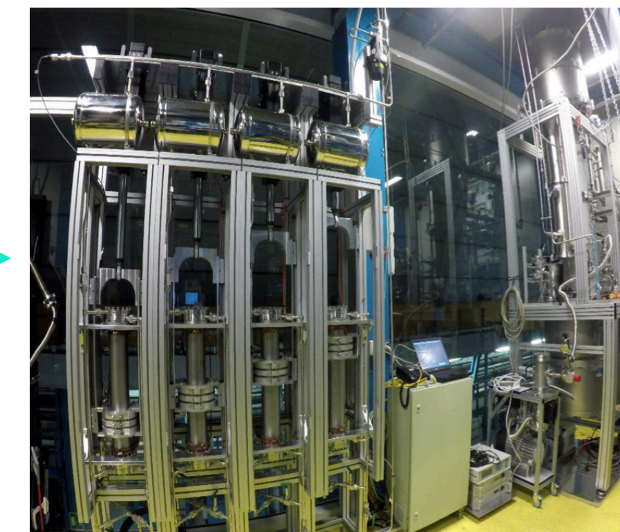
Radon distillation column Murra et al., JINST 17 P05037 (2022)
