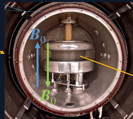
Measure spin-precession frequency of stored ultracold neutrons (UCN) under a constant magnetic field  $B_0$
