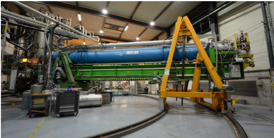
Fig. 9. The axion-helioscope concept. Axions are produced in the sun and travel towards the earth. In the presence of a transverse magnetic field in the helioscope (corresponding to the blue photon in the figure), the axions are converted into x-ray photons and detected. The energy spectrum of the x-ray photons corresponds to that of the axions produced in the sun.
