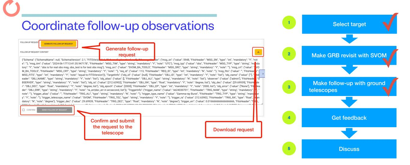
After completing the observation parameter of CGFT, BA need to generate the follow-up request. The parameters are automatically filled into the request. We recommend BA to check carefully before sending to the telescope.
