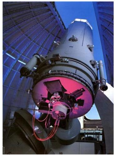
MISTRAL : a new spectrograph at Observatoire de Haute-Provence (France), permanently mounted on the T193cm telescope
