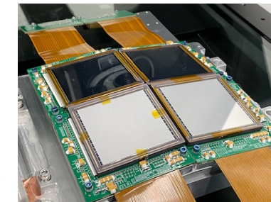
WXT mirror & CMOS detectors (1 module)
