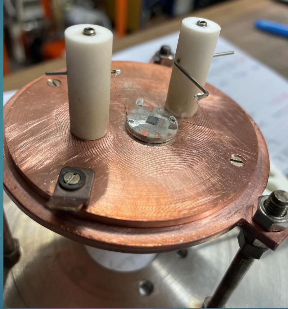
Wire connection used to apply an electric field through the sample
