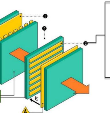
32 horizontal (vertical) gold strips of length 70 mm, width 1.85 mm, and thickness 50 nm representing the cathodes. The strips emit the secondary electrons. The signal (current from each strip) provide the horizontal (vertical) profile
