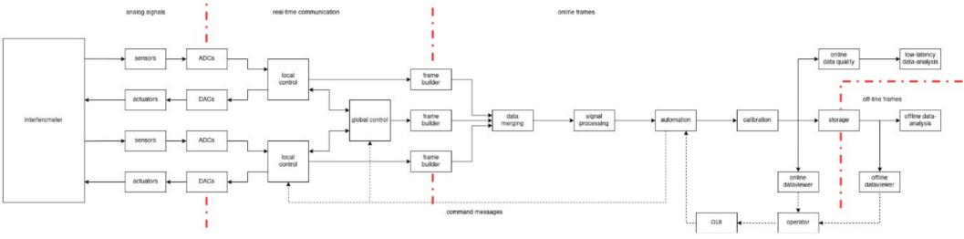
Analog signals of sensors/actuators converted to/from digital, sent around for digital realtime controls Fast signals **collected** by "frame builders" into chunks of data (0.1 to 1.0 s), then merged with slow data
