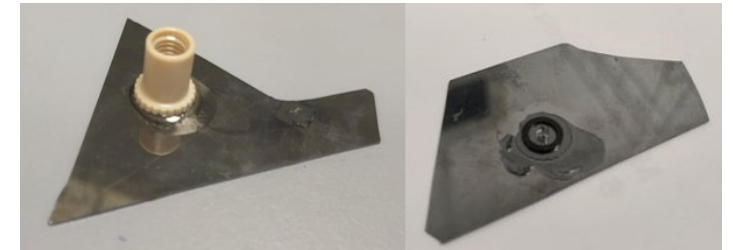
Commercial connection with glue P_{\text{max}} < 20 \text{ bar}
