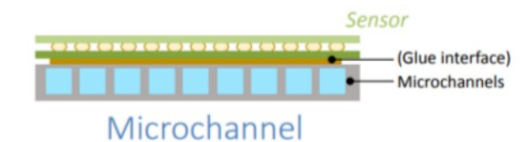
Multi micro-channels 0.2mm → TFM < 3 Kcm²/W
