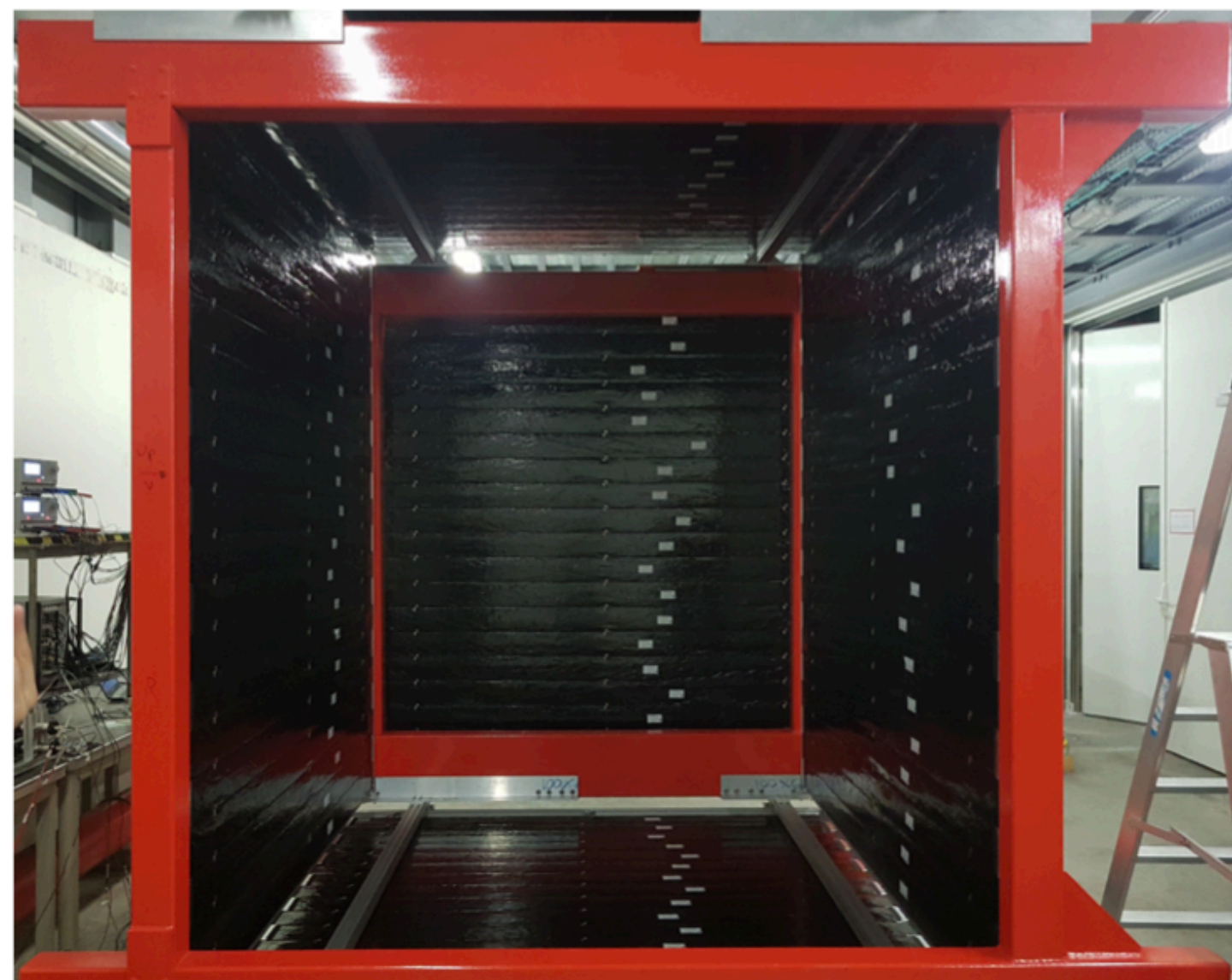
TOF panels assembled in ND280 basket prototype at CERN, June 2022
