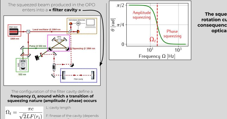
The squeezing ellipse rotation curve shape is a consequence of filter cavity optical behavior
