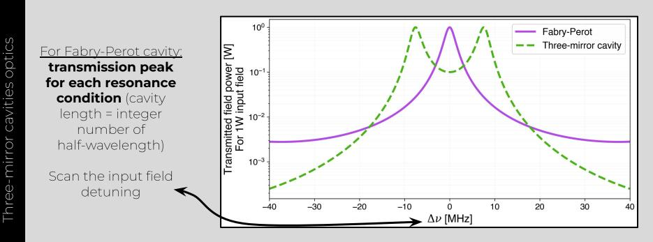
A <u>three-mirror cavity</u> can show off a <u>doubling of the</u> <u>transmission peak</u>
