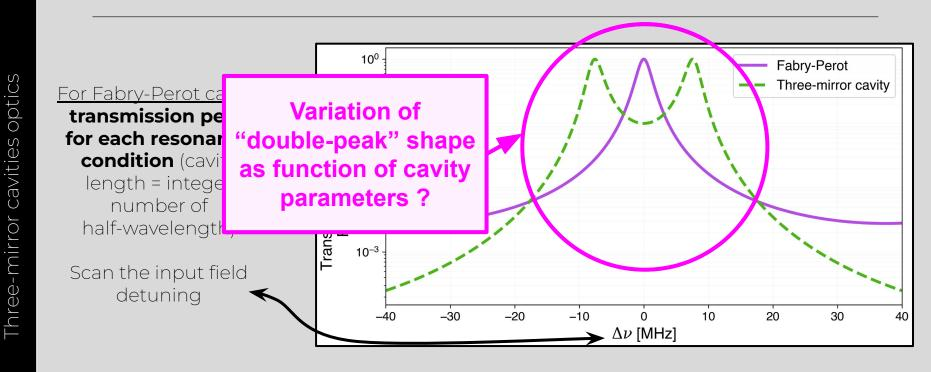
A <u>three-mirror cavity</u> can show off a <u>doubling of the</u> <u>transmission peak</u>
