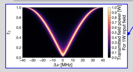
Second mirror transmissivity → symmetrical variation of space between maxima
