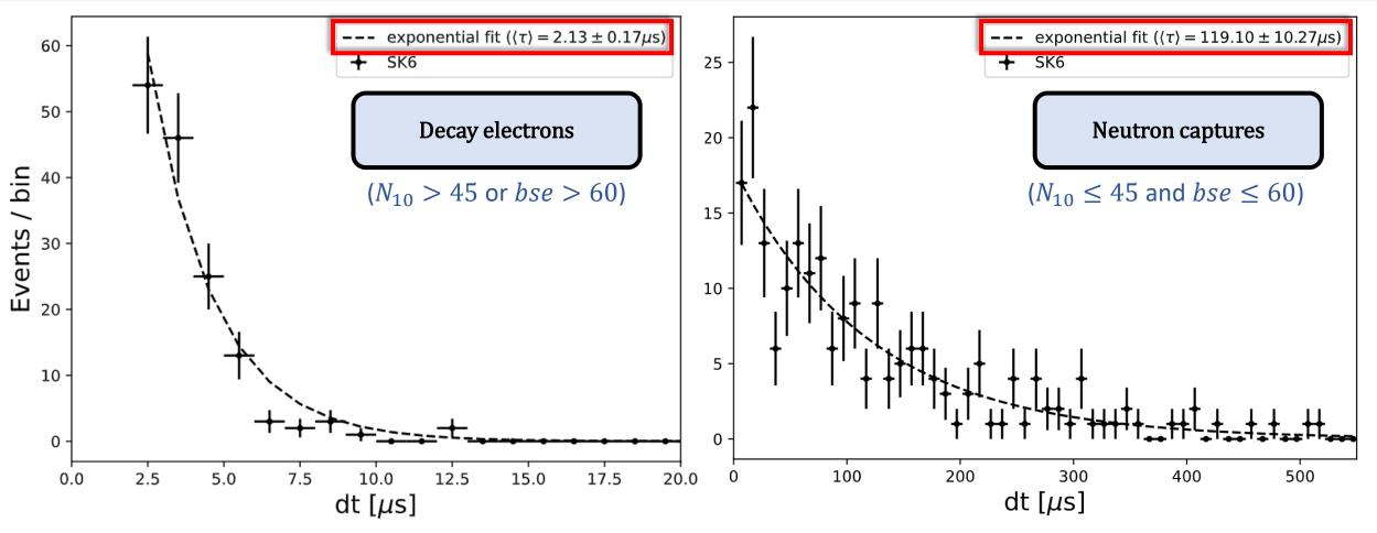
• **Decay-e sample** timing  $\tau = 2.1 \pm 0.2 \mu s$  **consistent** with  $\mu$ -decays.
