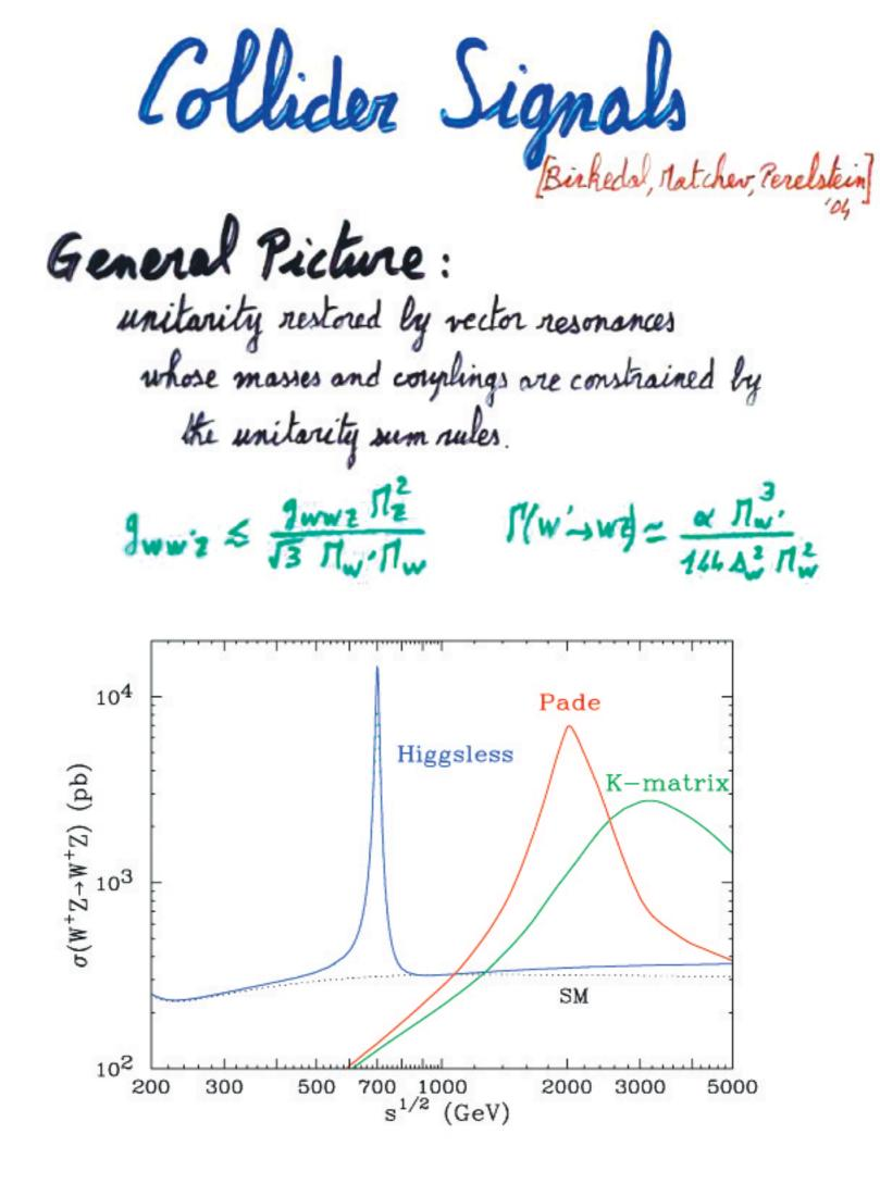
WZ elastic scattering cross sections in the SM (dotted), the Higgsless model (blue) and two technicolor-like models
