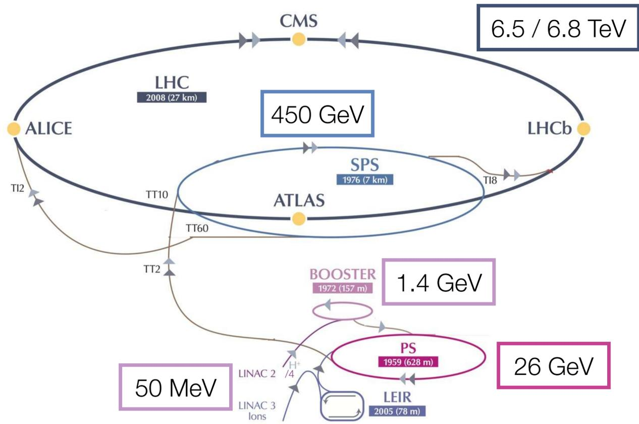
Located under the French-Swiss border, the **Large Hadron Collider** is the final piece of a staged acceleration chain allowing high luminosity **proton-proton** collisions.
