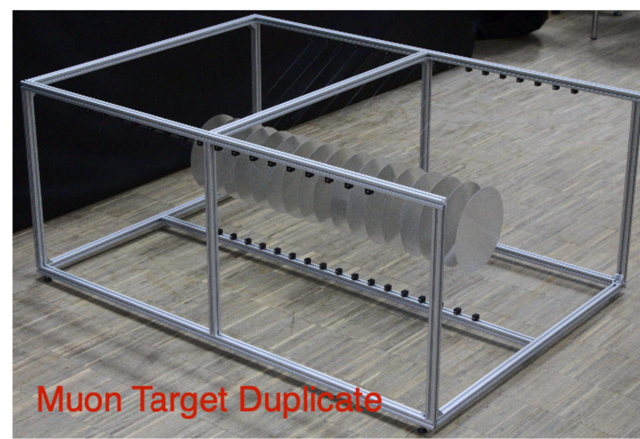
17 Al disks 100 mm radius, 200 μm thick Number of Signal Events
