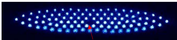
dark ion in capture trap ( \text{H}_2^+ or \text{H}_3^+ ) L. Hilico, J.-Ph. Karr et al. (LKB-Paris)
