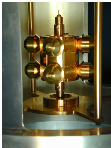
[Torsion pendulum used in Eöt-Wash experiments]
