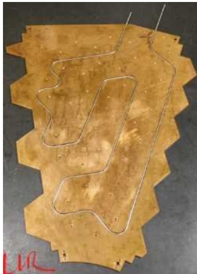
Pipe insertion on a cooling prototype
