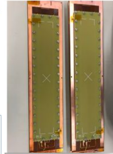
\mu -RWELL prototypes with 40 cm long strips
