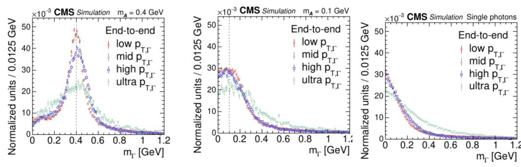
Using a CNN-based algorithm, reconstruct peak of 100 MeV particle. CMS granularity: 2.3 cm, IDEA Crystal: 1 cm IDEA Fiber: 2 mm Can probably improve on CMS result
