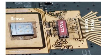
LGAD - 2x2 matrix wire-bonded to the input of the ASIC
