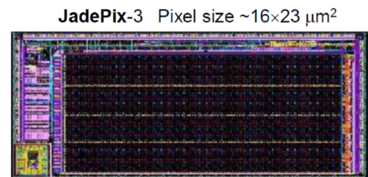
Tower-Jazz 180nm CIS process Resolution 5 microns, 53 \text{ mW/cm}^2
