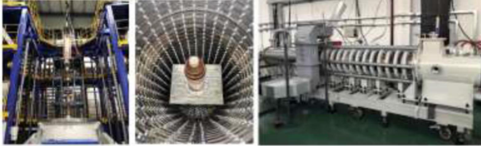
Klystron No. 1 Efficiency 65% (2020)
