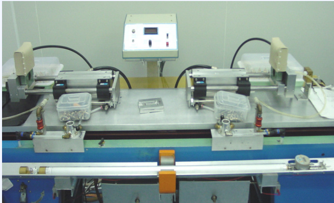
Assembling table & Wire tension measurement
