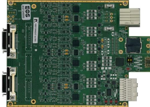
Input from pre-amplifiers by 10m MDR cables Requires 1 backplane with power distribution and 1 backplane with the 100 MHz clock distribution.
