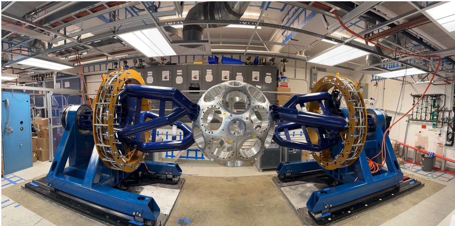
Support frames installed and aligned in the K-area in building 88
