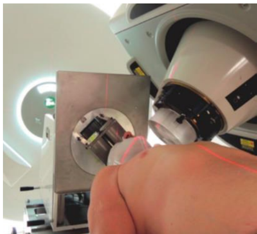
Knife-edge slit camera (IBA, Xie et al 2017) Tested in clinics
