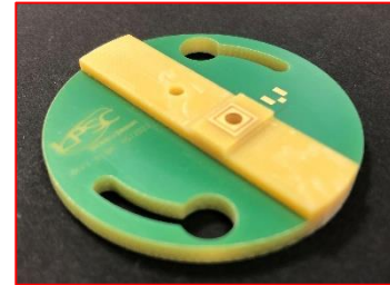
DéfiDiams sample holder - Produced by the Detector, Instrumentation and Electronics Departments at LPSC
